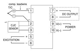
\*1. Attach the CJC sensor regardless of setting for cold junction compensation.
