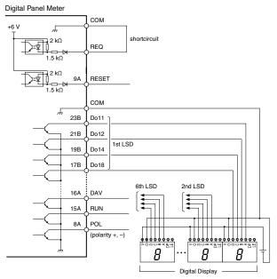
Use Special cable (model: HDR40) and Connector Terminal Block (model: CNT).
