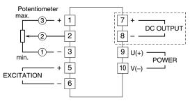
Note: The section enclosed by broken line is only with DC output option.
