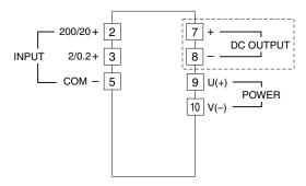
Note: The section enclosed by broken line is only with DC output option.
