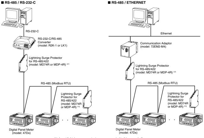
\*1. Insert lightning surge protectors recommended in this example if necessary.
