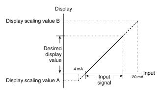
The next paragraph describes how to calculate the display scaling value A and B when the input is other than 4-20 mA DC.
