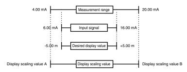
Calculate the display scaling value A and B with the following formulas.
