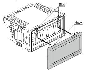
(2) Push the panel hook into the case downside slots of the unit.
