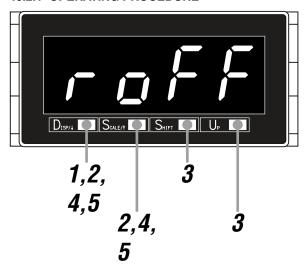
Hold down Disp/↑ button for 3 seconds or more to move on to **Display Setting Mode.**
