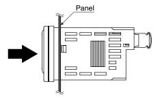
(3) Push the mounting brackets into the grooves on both sides of the rear module, until they hit the panel's rear side.
