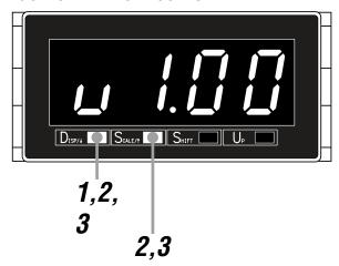
Hold down Disp/↑ button for 3 seconds or more to move on to **Display Setting Mode.**
