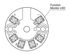
■INPUT MONITOR: The input 0 – 100% is converted into a combination of 1-second (1 unit) and 0.25-second (0.2 unit) cycled pulses. 1 unit corresponds to 25%, while 0.2 unit corresponds to 5%. 0% equals to 1 unit, while 100% corresponds to 5 units. The input % is represented in the total number of 1-unit pulses and 0.2-unit pulses, repeated in the sequence of '1-unit pulses —> 0.2-unit pulses —> OFF for 1 second or more.'
