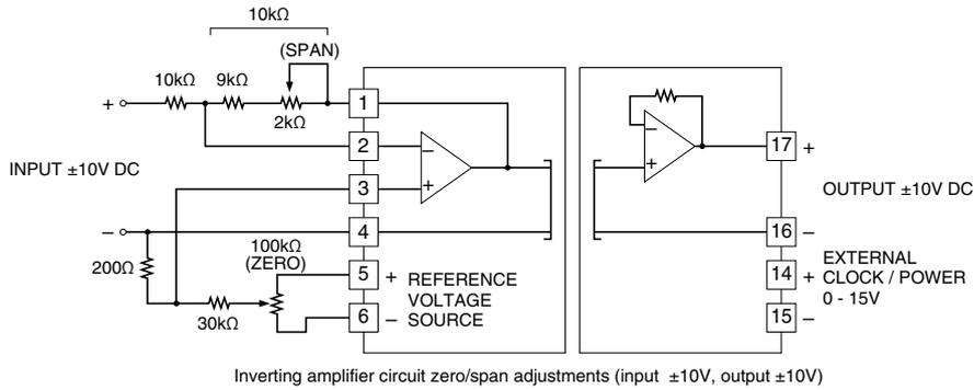
For an inverting amplification with external adjustments, when the combined resistance of the span adjustment and 9kΩ is 10kΩ, the gain is  $-(10k\Omega / R_2) \times V_{IN}$ . With the span adjustment (2kΩ), the output is configurable. The zero is adjustable with a reference voltage source of ±15V DC and the attenuation of 200Ω and 30kΩ.
