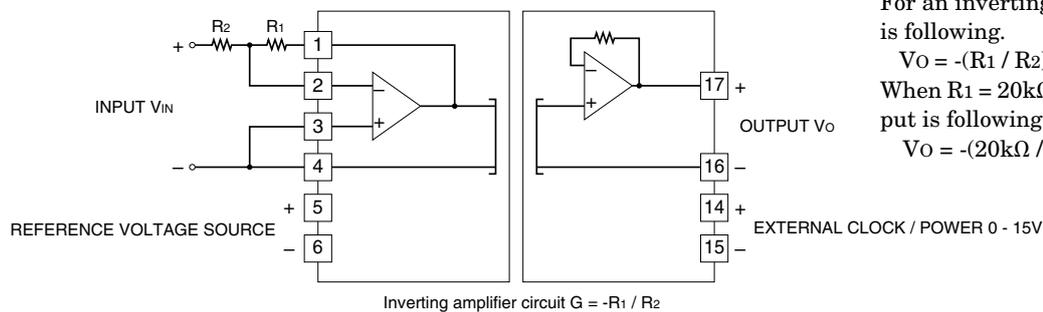
For an inverting amplification the output is following.
