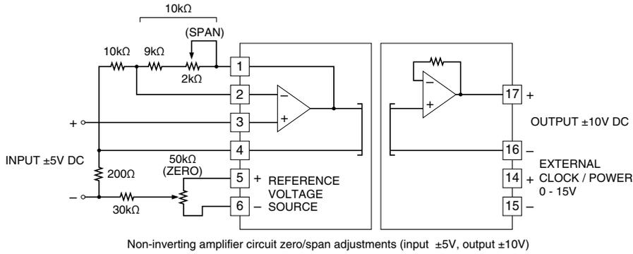
For a non-inverting amplification with external adjustments, when the combined resistance of the span adjustment and 9kΩ is 10kΩ, the gain is  $(1 + 10k\Omega / R_1) \times V_{IN}$ . With the span adjustment (2kΩ), the output is configurable. The zero is adjustable with a reference voltage source of ±15V DC and the attenuation of 200Ω and 30kΩ.
