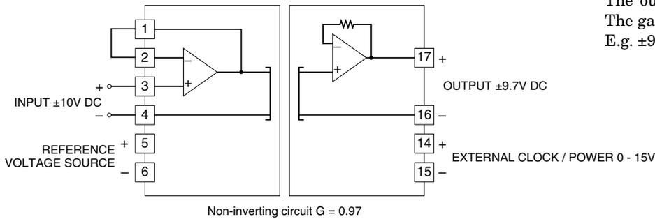
The output is proportional to the input. The gain is 0.97. E.g.  $\pm 9.7V$  DC for  $\pm 10V$  DC input.
