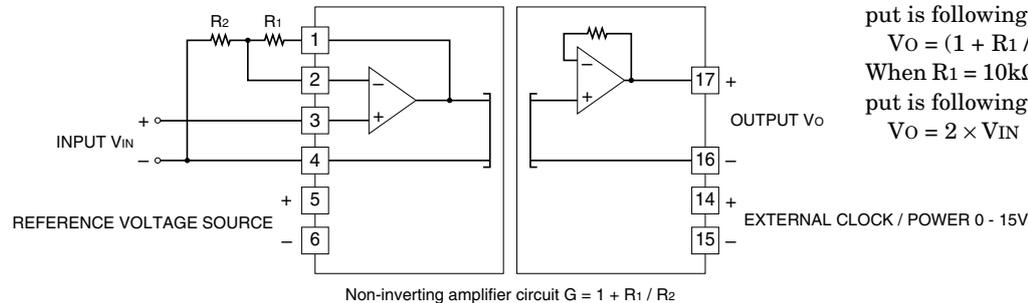
For a non-inverting amplification the output is following.
