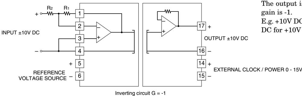
The output is inverted to the input. The gain is -1. E.g. +10V DC for -10V DC input and -10V DC for +10V DC input.
