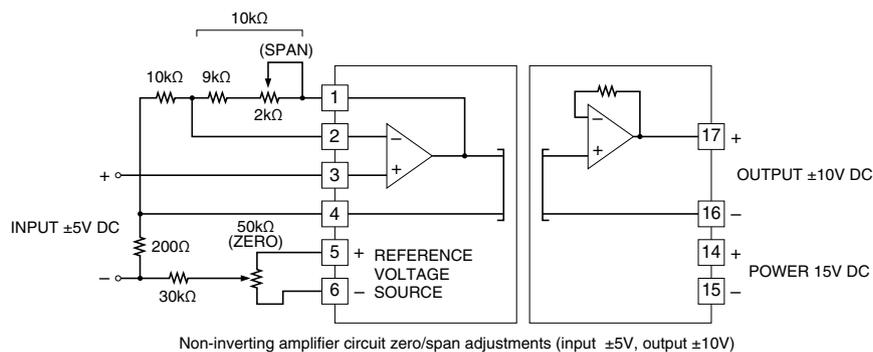
For a non-inverting amplification with external adjustments, when the combined resistance of the span adjustment and  $9k\Omega$  is  $10k\Omega$ , the gain is  $(1 + 10k\Omega / R_1) \times V_{IN}$ . With the span adjustment ( $2k\Omega$ ), the output is configurable. The zero is adjustable with a reference voltage source of  $\pm 15V$  DC and the attenuation of  $200\Omega$  and  $30k\Omega$ .
