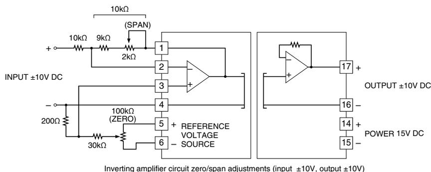
For an inverting amplification with external adjustments, when the combined resistance of the span adjustment and  $9k\Omega$  is  $10k\Omega$ , the gain is  $-(10k\Omega / R_2) \times V_{IN}$ . With the span adjustment ( $2k\Omega$ ), the output is configurable. The zero is adjustable with a reference voltage source of  $\pm 15V$  DC and the attenuation of  $200\Omega$  and  $30k\Omega$ .
