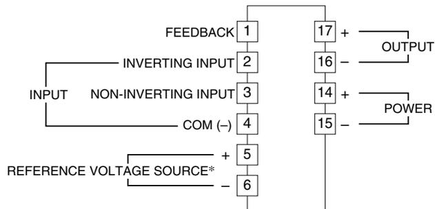
Note. The reference voltage source is common to the COM (-), terminal 4.
