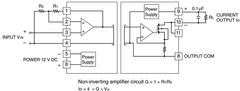
For a non-inverting amplification the output is following.
