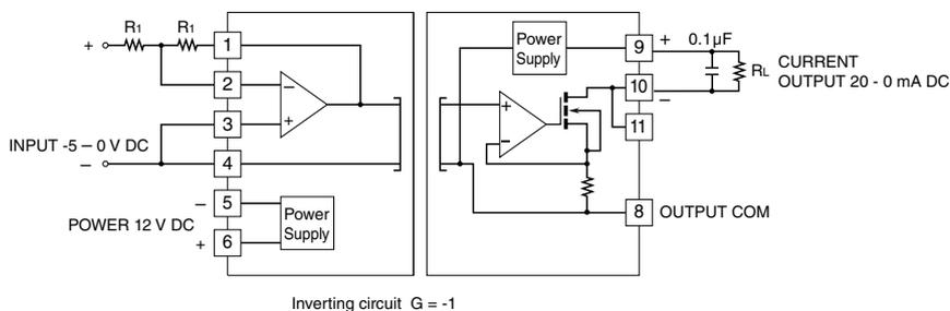
The output is inverted to the input.
