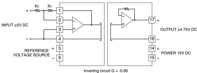
The output is inverted to the input. The gain is -0.95.
