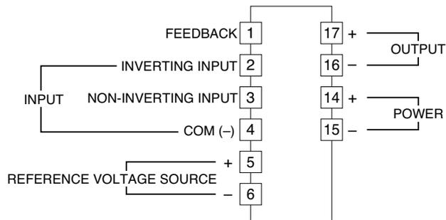
Note. The reference voltage source is common to the COM (-), terminal 4.
