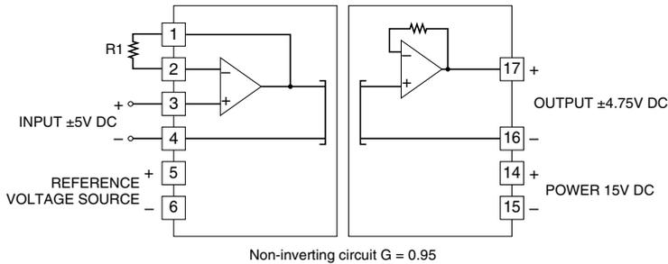
The output is proportional to the input. The gain is 0.95.
