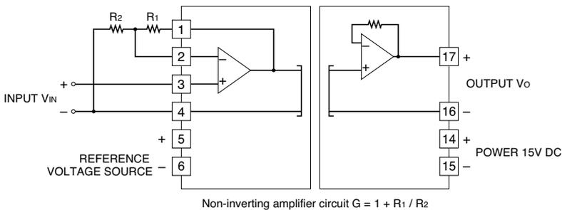
For a non-inverting amplification the output is following.
