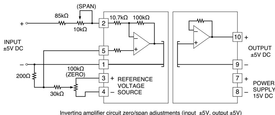
For an inverting amplification with external adjustments, when the combined resistance of the span adjustment and  $85k\Omega$  is  $89.3k\Omega$ , the gain is  $-V_{IN}$ . With the span adjustment ( $2k\Omega$ ), the output is configurable. The zero is adjustable with a reference voltage source of  $\pm 7.5V$  DC and the attenuation of  $200\Omega$  and  $30k\Omega$ .
