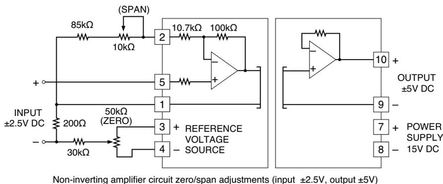
For a non-inverting amplification with external adjustments, when the combined resistance of the span adjustment and  $85k\Omega$  is  $89.3k\Omega$ , the gain is  $2 \times V_{IN}$ . With the span adjustment ( $2k\Omega$ ), the output is configurable. The zero is adjustable with a reference voltage source of  $\pm 7.5V$  DC and the attenuation of  $200\Omega$  and  $30k\Omega$ .
