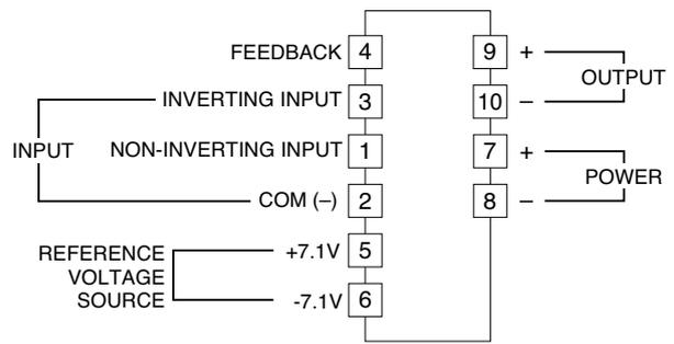
Note. The reference voltage source is common to the COM (-), terminal 2.
