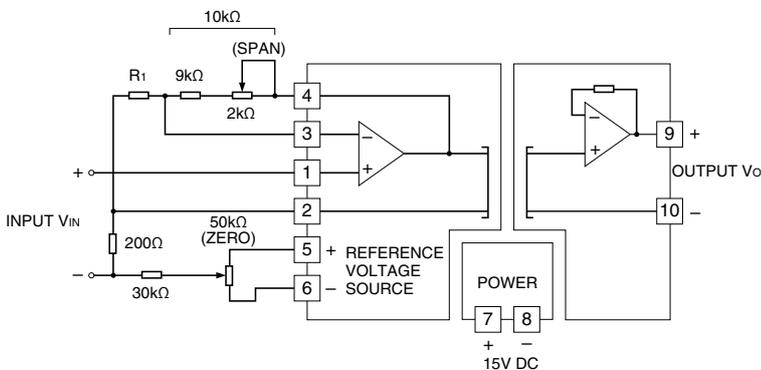
For a non-inverting amplification with external adjustments, when the combined resistance of the span adjustment and 9kΩ is 10kΩ, the gain is  $(1 + 10k\Omega / R_1) \times V_{IN}$ . With the span adjustment (2kΩ), the output is configurable. The zero is adjustable with a reference voltage source of  $\pm 7.1V$  DC and the attenuation of 200Ω and 30kΩ.
