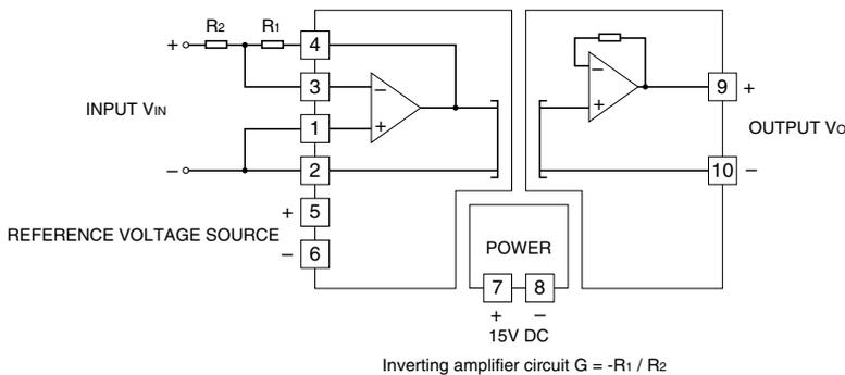
For an inverting amplification the output is following.
