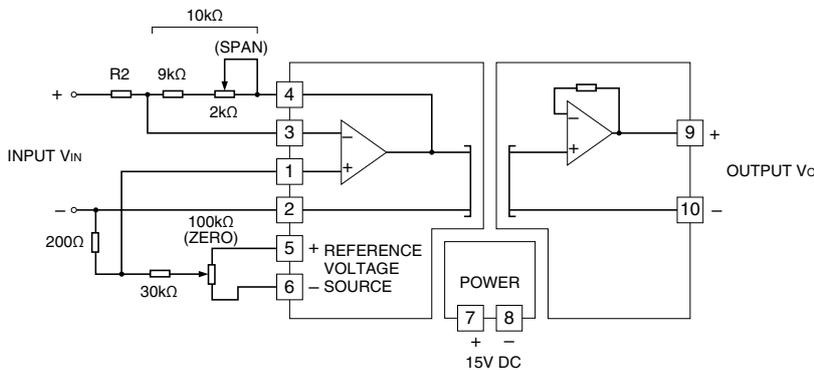
For an inverting amplification with external adjustments, when the combined resistance of the span adjustment and 9kΩ is 10kΩ, the gain is  $-(10k\Omega / R_2) \times V_{IN}$ . With the span adjustment (2kΩ), the output is configurable. The zero is adjustable with a reference voltage source of  $\pm 7.1V$  DC and the attenuation of 200Ω and 30kΩ.
