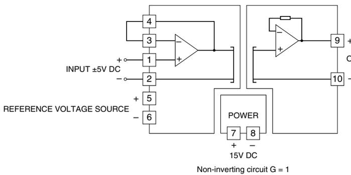
The output is proportional to the input. The gain is 1.
