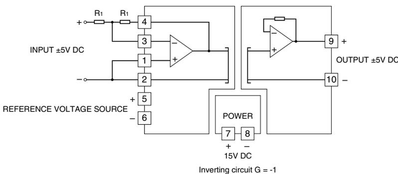
The output is inverted to the input. The gain is -1.
