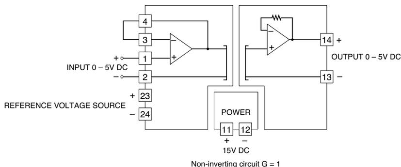
The output is proportional to the input. The gain is 1.
