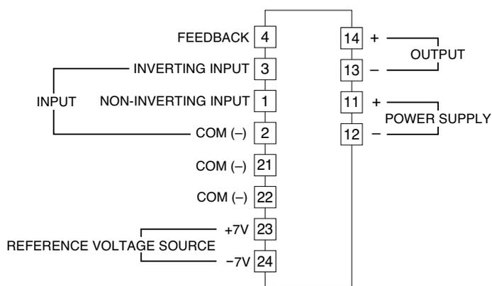
Note. The reference voltage source is common to the COM (-), terminals 2, 21 and 22.
