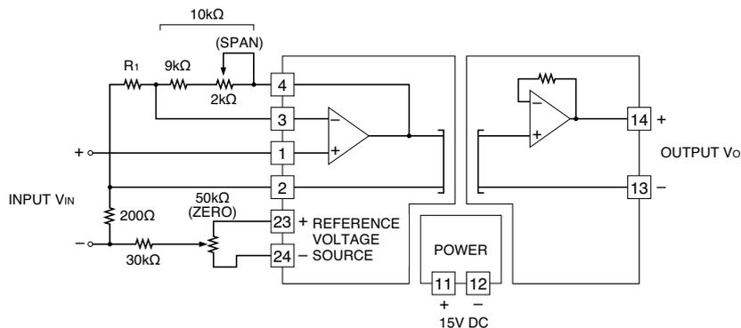
For a non-inverting amplification with external adjustments, when the combined resistance of the span adjustment and 9kΩ is 10kΩ, the gain is  $(1 + 10\text{k}\Omega / R_1) \times V_{IN}$ . With the span adjustment (2kΩ), the output is configurable. The zero is adjustable with a reference voltage source of  $\pm 7.0\text{V DC}$  and the attenuation of 200Ω and 30kΩ.
