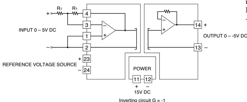
The output is inverted to the input. The gain is -1.
