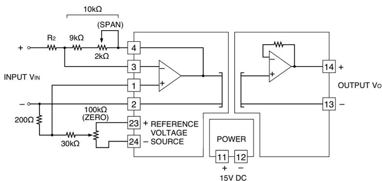
For an inverting amplification with external adjustments, when the combined resistance of the span adjustment and 9kΩ is 10kΩ, the gain is  $-(10\text{k}\Omega / R_2) \times V_{IN}$ . With the span adjustment (2kΩ), the output is configurable. The zero is adjustable with a reference voltage source of  $\pm 7.0\text{V DC}$  and the attenuation of 200Ω and 30kΩ.
