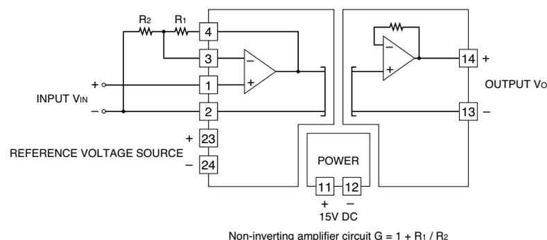
For a non-inverting amplification the output is following.
